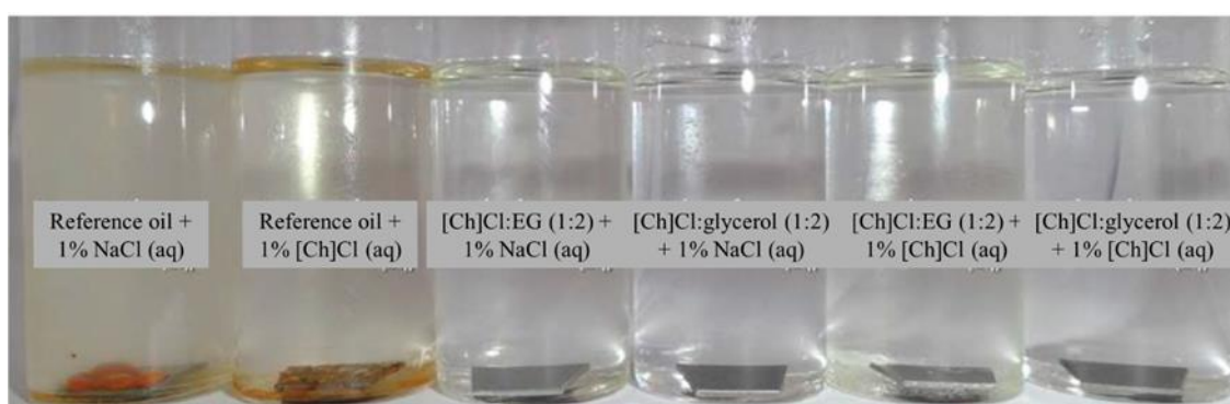
Figure 1.11. Corrosion experiments of mild steel after 2 weeks of immersion in the reference oil and the DES containing 1% NaCl (aq) and 1% [Ch]Cl (aq). Adapted from reference [112].
