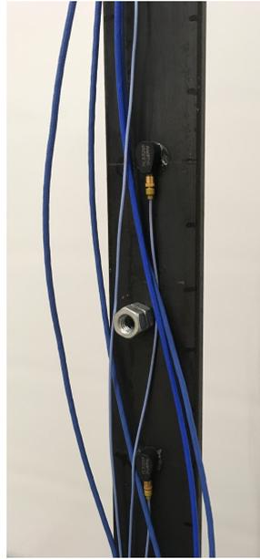
**Figure 5.3.** Close-up of the damage placed on the beam used in the experimental application.
