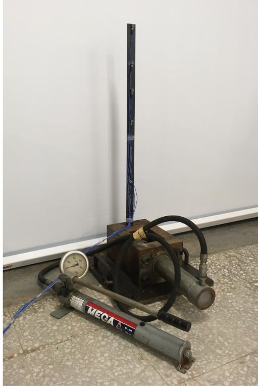
**Figure 5.1.** Beam used in experimental application, with the sensor placements and the hydraulic press to fix one of its edges.
