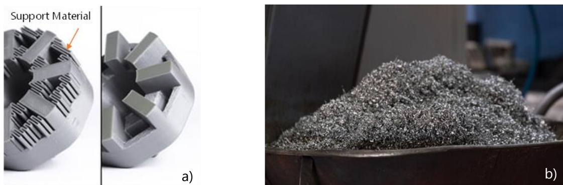
Figure 2.10 - Wasted material a)- 3D printed support; b)- Metal Shavings [35], [36].
