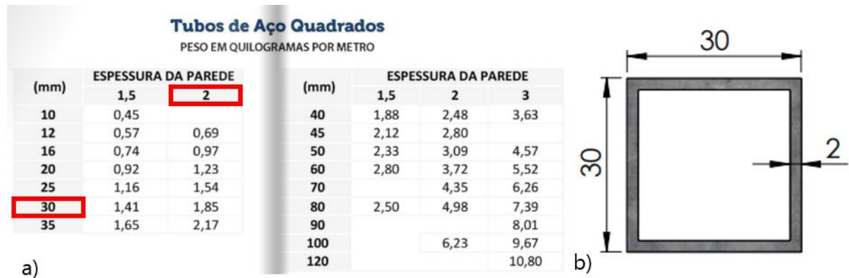
Figure 5.5 - a) Profiles sizes and weight; b) Chosen dimensions in millimeters [82].
