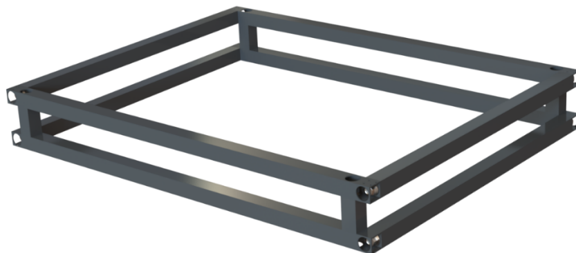
Figure 5.6 - 3D render of the main frame subassembly.
