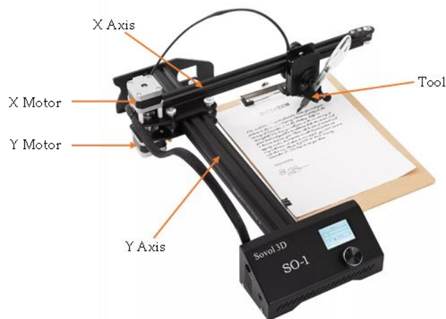
Figure 2.1 - Two axes CNC writing machine [13].
