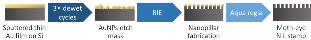
Fig. 2.2 – Schematic representation of the ME master stamp process-flow.
