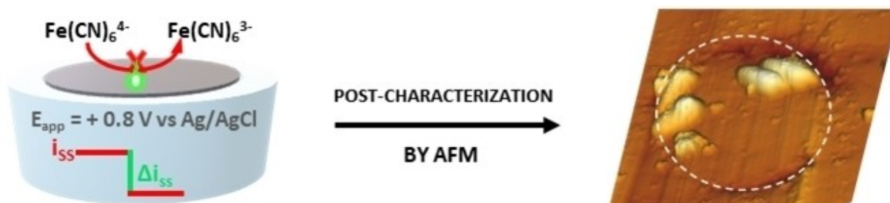
Figure 1. Single electrochemical impacts of Shewanella oneidensis MR-1 onto an ultramicroelectrode (UME) polarized at the oxidation potential (+0.8 V vs Ag/AgCl) of the ferrocyanide redox probe in solution and post-characterization of the living bacteria adsorption onto the UME surface by atomic force microscopy.
