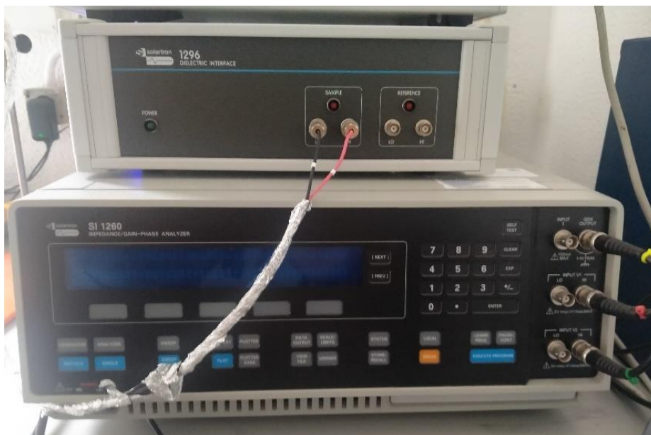
Figure 3.4: Impedance spectrometer instruments. 1296A dielectric interface on the 1260A impedance analyzer
