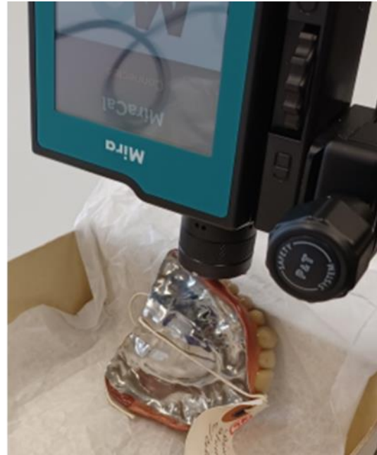
Figure A2.4. Raman MIRA DS analysis of the swaged gold and celluloid dental plate JUSTI 21 from NMD (left) and of the vulcanized rubber and Vitallium alloy denture MG.291116.0046 from NMAH (right), using the 3mm distance objective set up.
