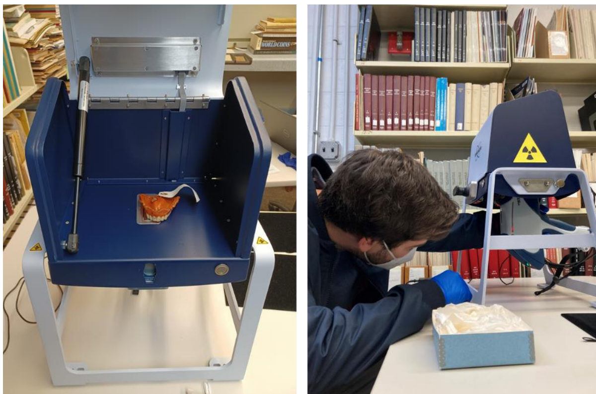
Figure A2.6. Right, celluloid denture inside the X-ray fluorescence spectrometer S1 Titan analysis chamber. The analysis area where the x-ray beam interacted with the object is beneath the denture. The chamber lid was closed for analysis. Left, different view where it is possible to see the X-ray fluorescence spectrometer S1 Titan beneath the analysis chamber. The trigger had to be pressed during the analysis; the time corresponding to the acquisition time.
