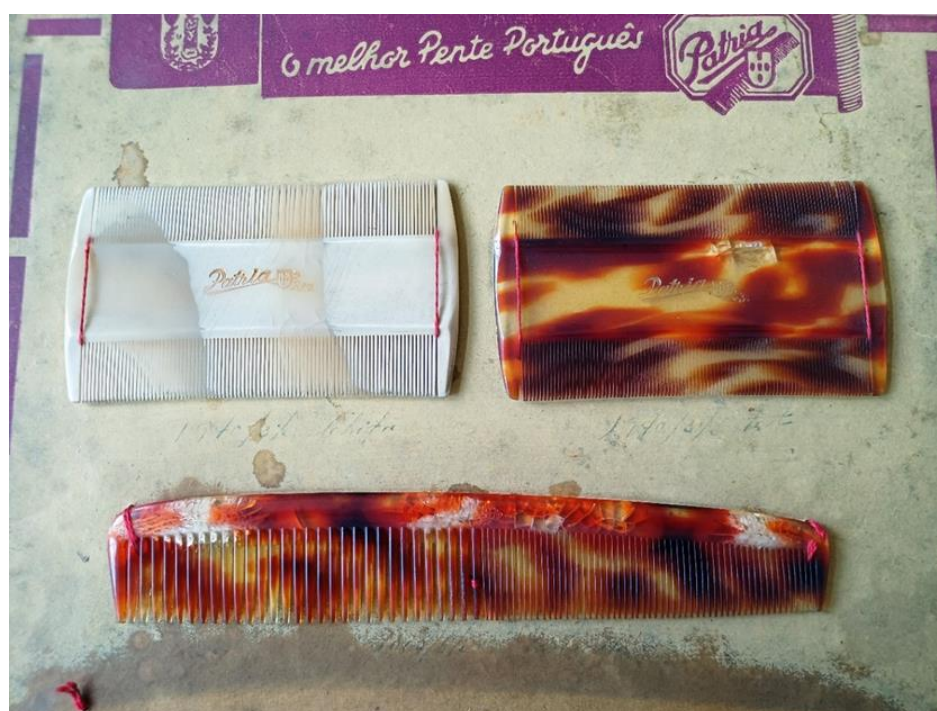
Figure A3.9. Celluloid combs from the of “Fábrica de Plásticos Pátria” from the collection of Sociedade Martins Sarmento, Guimarães, where it is possible to see the cracking pattern of extreme celluloid degradation.
