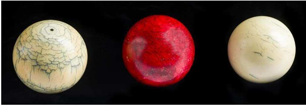
Figure A1.28. Photograph of the NMAH's ivory billiards balls, dated from 1875-1920 (ID Number CL.329507). The dimensions and weight of left and right billiard balls were measured: 57mm and 174.2g; 54mm and 143.8g, respectively.
