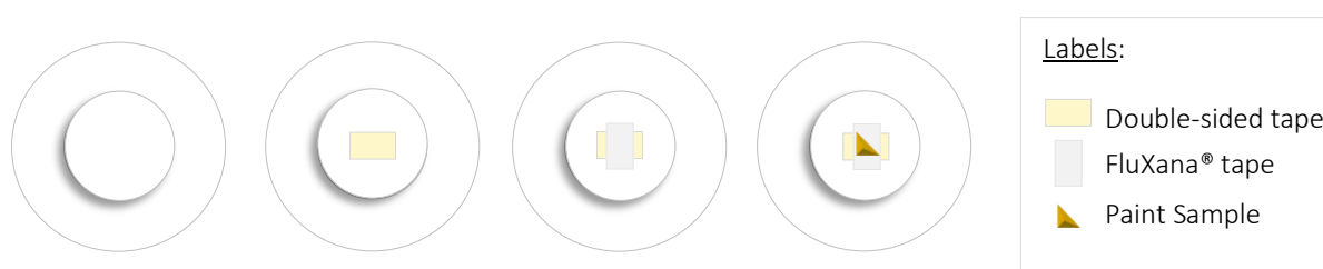
Scheme C.1: Sequence of steps to adhere the sample on the base of the embedding mould.
