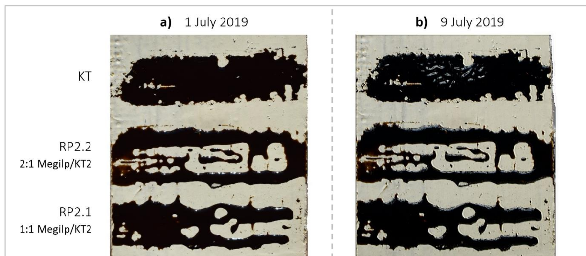
Figure 5.3: KT and RP product applied on a 14-year-old reconstruction of a W&N oil ground. a) immediately after being painted on the 1st of July and b) after a week.
