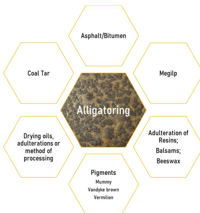
Scheme 1.1: Scheme of the materials mention in the literature as possible causes for Alligatoring.
