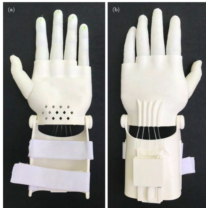
Figure 7.2: Main developed prosthesis by Ana Oliveira's thesis [63]: (a) anterior view; (b) posterior view.
