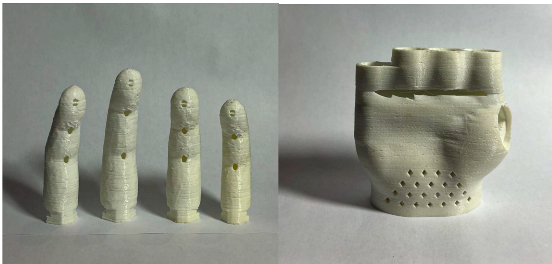
(a) Final fingers vertically printed.
