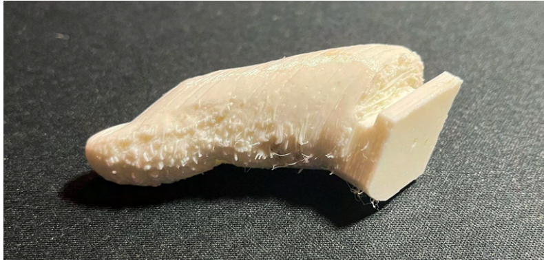
Figure 7.48: Bottom view of the printed thumb for the final prosthesis prototype.
