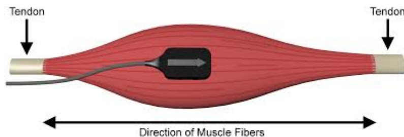
Figure 4.3: Diagram of ideal electrode placement in regards to the orientation of the muscle fibers [55].
