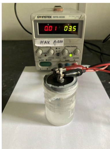
Figure 4.9: Photograph of the setup used for the electrodeposition method. Red electrode - anode (Graphite); Black electrode - cathode (Mg alloy)
