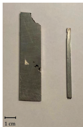
Figure 4.3: Photograph of part of a treated printed wall (left) and a sliced piece used for the study (right)
