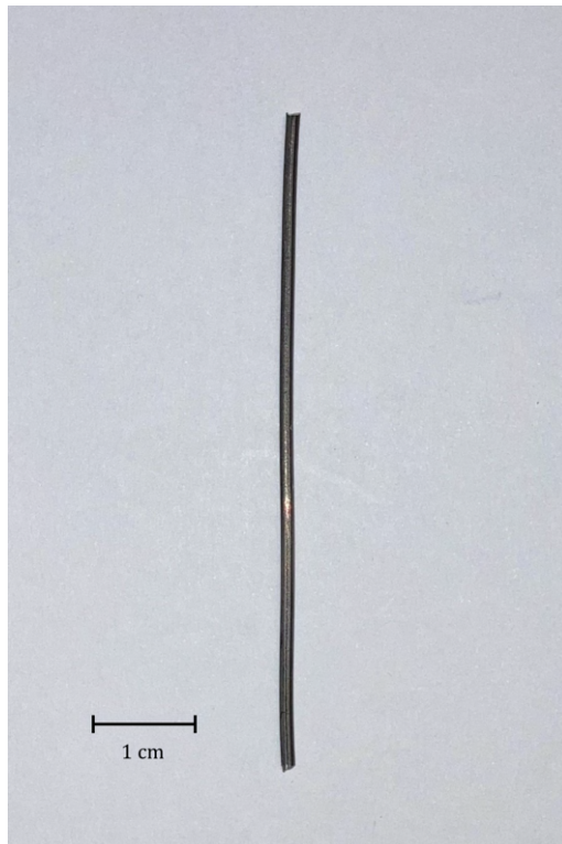
Figure I.1: Photograph of the commercial wire AZ61A, used to print the WAAM substrates
