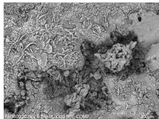
Figure 5.41: SEM of a WAAM printed Mg commercial alloy AZ61A after a CV experiment in neutral pH, with a deposition of 3.5 V for 2h
