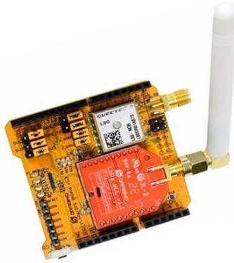
Figura 3.7: Dragino LoRa/GPS *Shield*.
