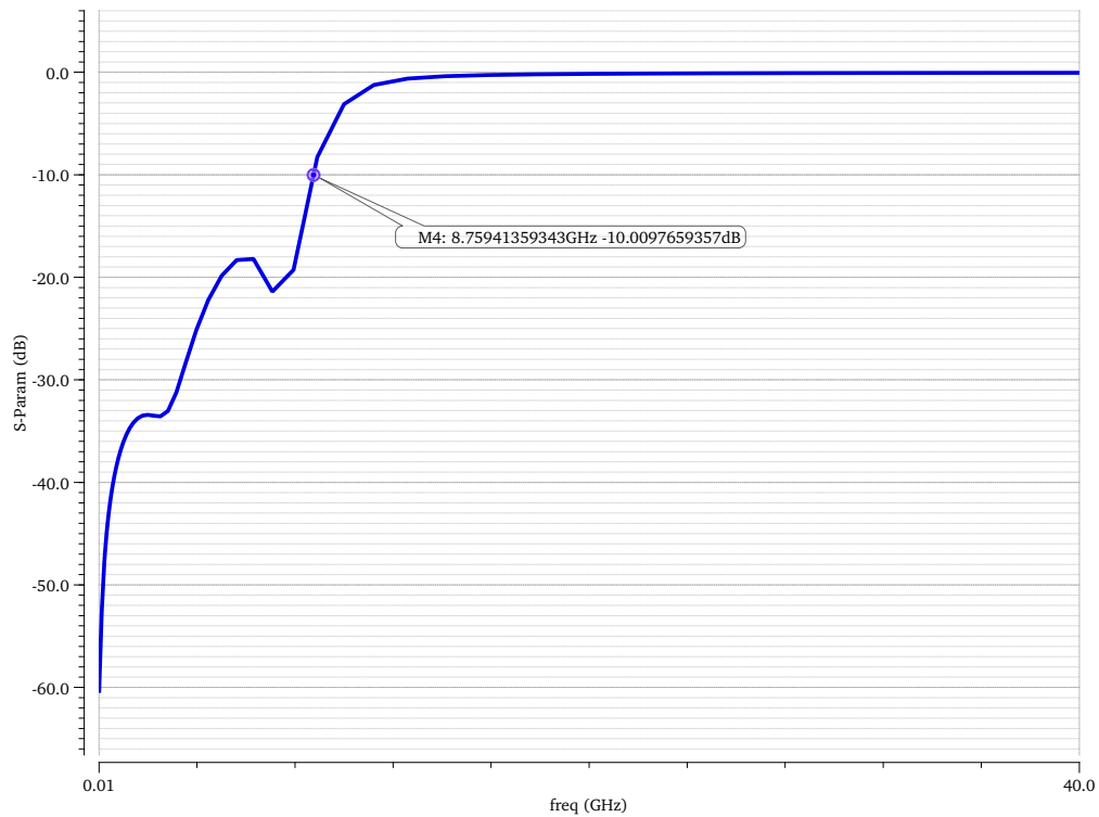
Figure 5.34: Push-pull frequency response in Cadence
