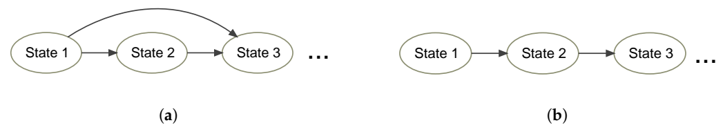
Figure 1. A fully dependent BN (a) and a BN respecting the Markov property (b).
