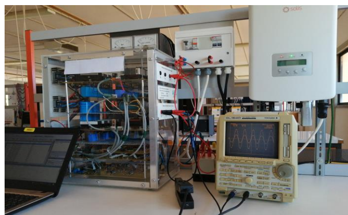
Figure 6. Prototype of the implemented solar inverter testing system.
