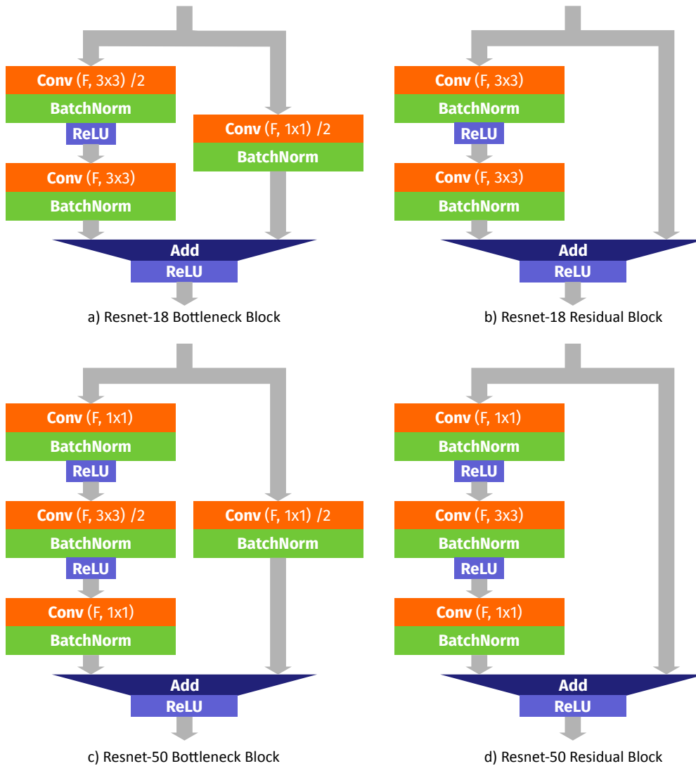
Figure 2: Schema of the building blocks of a residual network: the bottleneck block that usually downsamples the input by a factor of 2 using convolutions with stride, indicated with “/2” for ResNet-18 (a) and ResNet-50 (c), and the residual block for ResNet-18 (b) and ResNet-50 (d). Size of convolution kernels is indicated as, e.g., 3 \times 3 , and the letter F stands for the number of filters, which varies from one layer to another.
