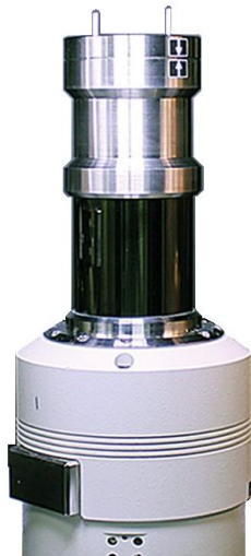
Tensile and compression stage DEBEN CT5000RT Up to 5 kN
