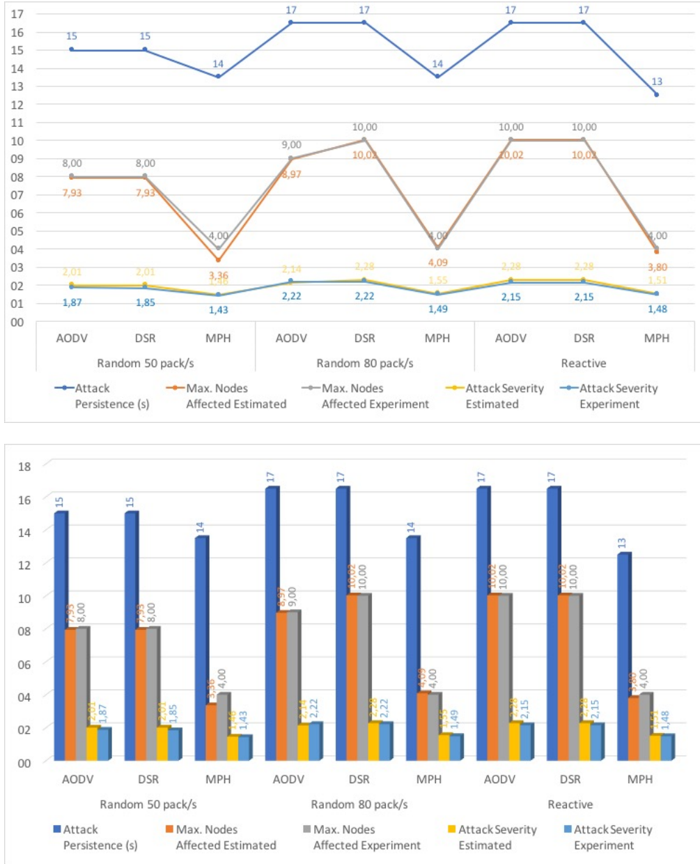
Fig. 5. Results obtained from simulations when the jammer node is in the middle of the topology. It is included the results for the three protocols (AODV, DSR and MPH), and three different attacks (random jamming attacks at 50 packets/s and 80 packets/s; and reactive jamming).
