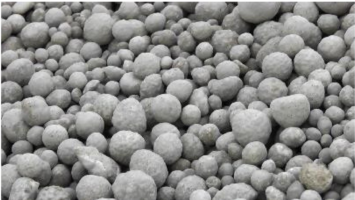
Figure 2. Manufactured carbonated aggregate <14 mm (courtesy of Carbon8 Systems, Ltd.).
