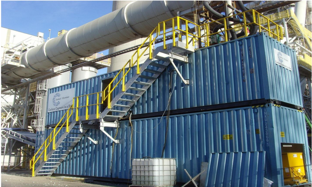
Figure 4. Mobile plant for manufacture of carbonated aggregates (courtesy of Carbon8 Systems, Ltd).
