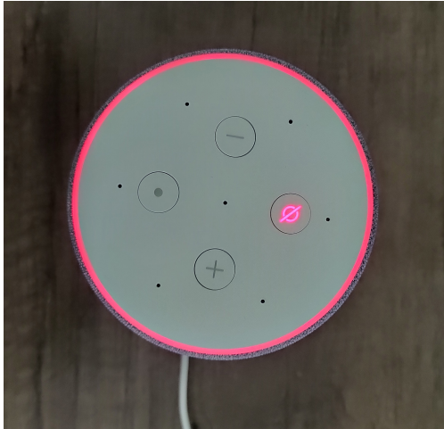
Figure 3.5: How to mute Amazon Echo? Echo’s LED light turns red while the mic is off.
