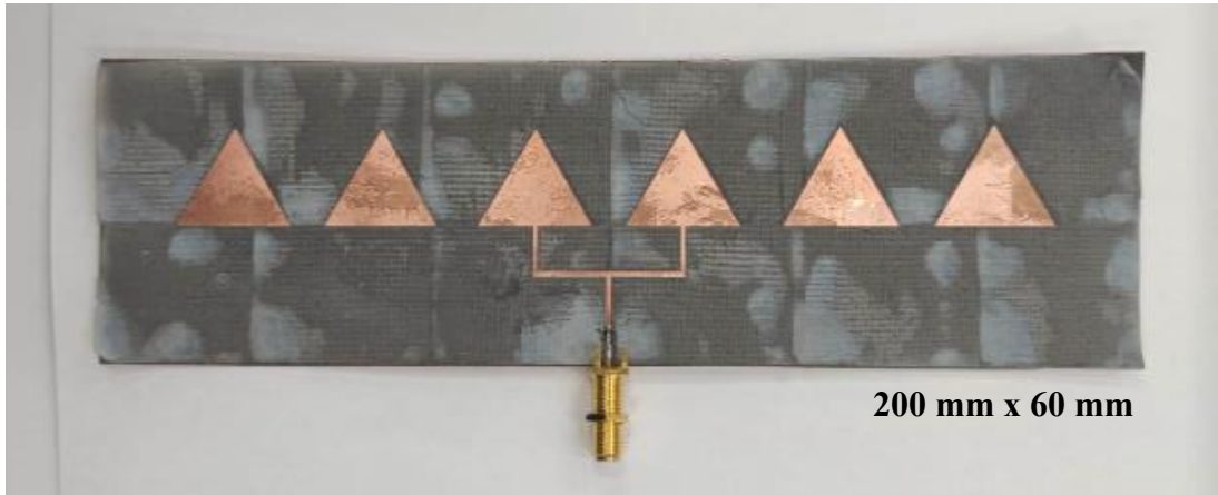
Figure 4.2 Fabricated 1st Approach: Single-plane folded patch.
