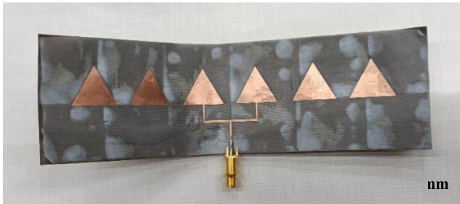
Figure 4.4 Fabricated 1st Approach: Single-plane folded patch when folds.
