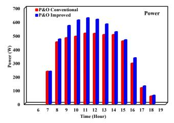
Figure 9. The output current, voltage, and maximum output power of the conventional and improved P&O.
