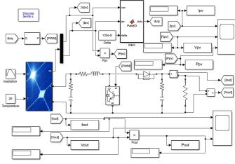
Figure 7. The block diagram of P&O MPPT controller.
