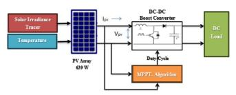
Figure 1. The block diagram of the proposed IoT and P&O system.
