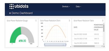
Figure 8. The ubidots live visualization of the measured solar power irradiance using the proposed IoT system.
