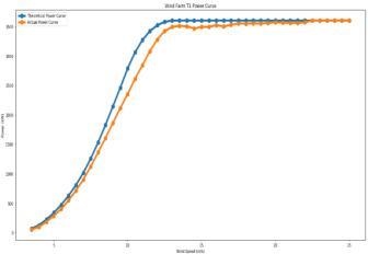
Figure 4. Wind Farm Power Curve
