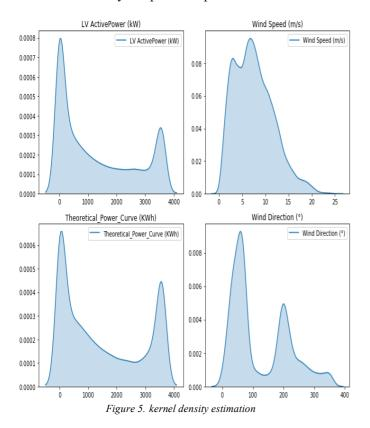
A grid of subplots is presented in Figure 5, the data distribution using kernel density estimation (KDE) plots for each column in the dataset. Each subplot represents the KDE plot for a specific column of the dataset. KDE plots are useful for understanding the shape and distribution of data, offering
