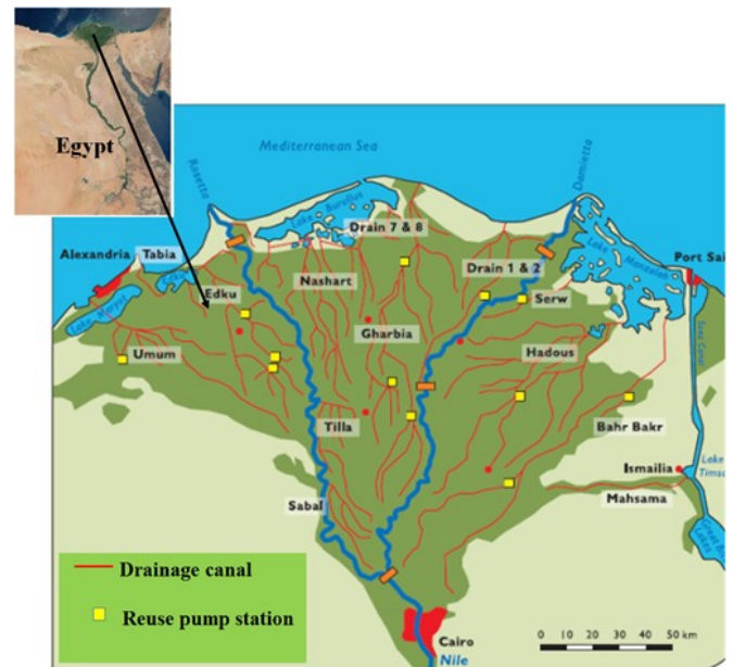
Figure 6. Drainage system in Delta
