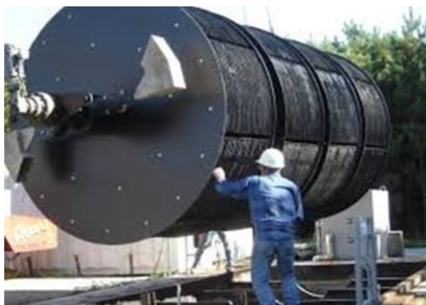
Figure 3. Rotating biological contractors.
