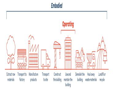
Fig.5: Lifecycle of a building (Source: BIM Corner)
