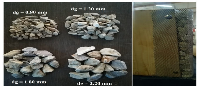
Figure 3. The fill material of the gabion basket.
