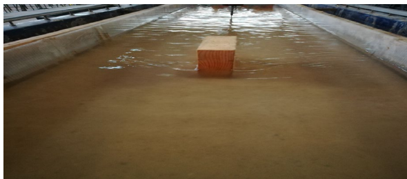
Figure 2. A modeled rectangular bridge pier at the considered laboratory flume.
