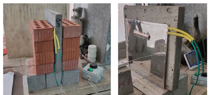
Figure 11. Testing samples of wall claddings (right) with bricks (left) [Authors].
