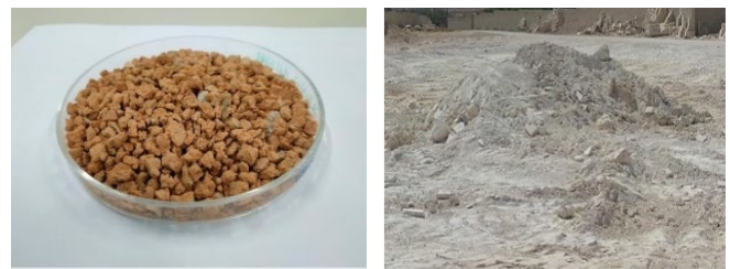
Figure 3. Brick waste (left) marble dust (right) [11].
