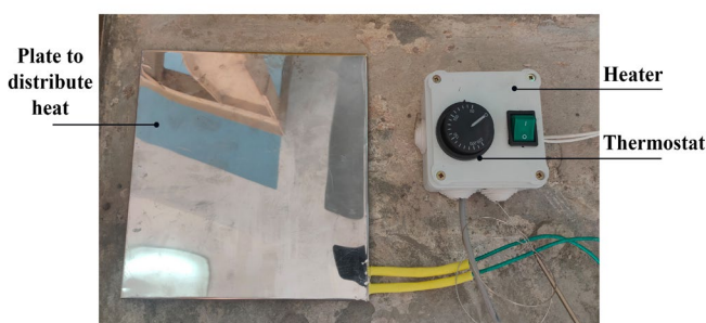
Figure 9. Apparatus used to conduct the experiment [Authors].
