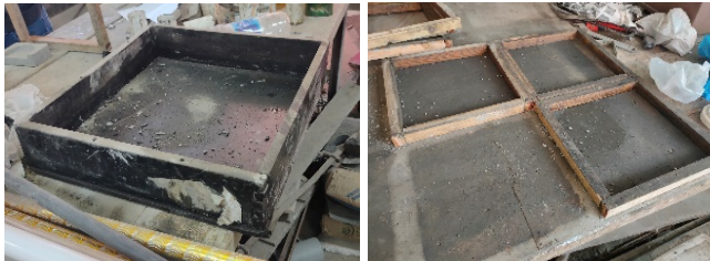
Figure 5. Steel form (left) wooden form (right) [Authors].
