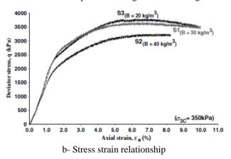
Figure 4. Effect of bentonite on plastic concrete behavior [29].
