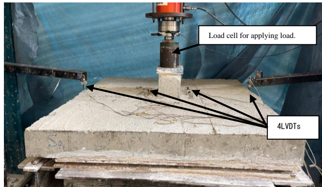
(a) Instrumentation at upper surface
