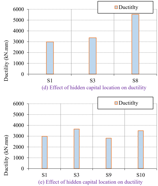
Figure 15. Effect of various parameters on ductility of slabs.
