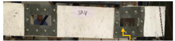
(c) Plate buckling
