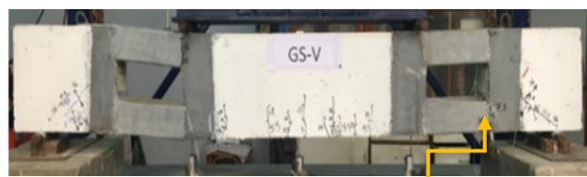
(a) Debonding of GFRP
