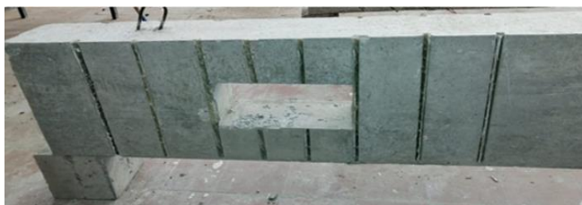
(a) Preparation of Grooves around the opening
