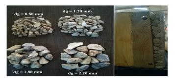
Figure 3. The fill material of the gabion basket.
