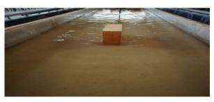
Figure 2. A modeled rectangular bridge pier at the considered laboratory Flume.
