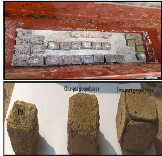
Figure 5. The physical appearance of geopolymer and PC samples after the exposure to 5% sulfuric acid.
