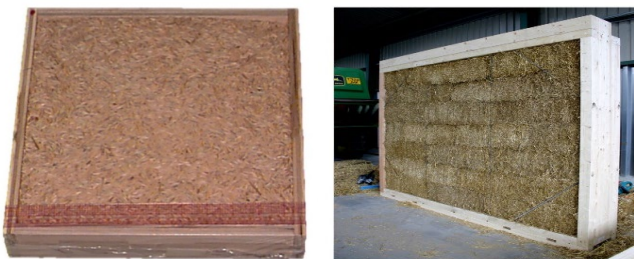
Figure 1. Wall claddings made of rice waste (left) and straw bale (right) [6], [7].
