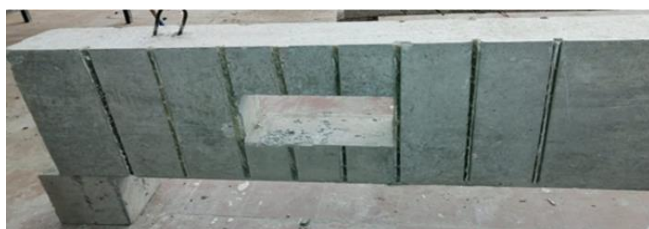
(a) Preparation of Grooves around the opening
