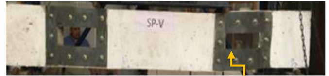
(c) Plate buckling
