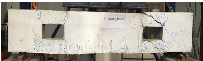
Figure 12. Crack pattern and failure mode of the control beam with opening
