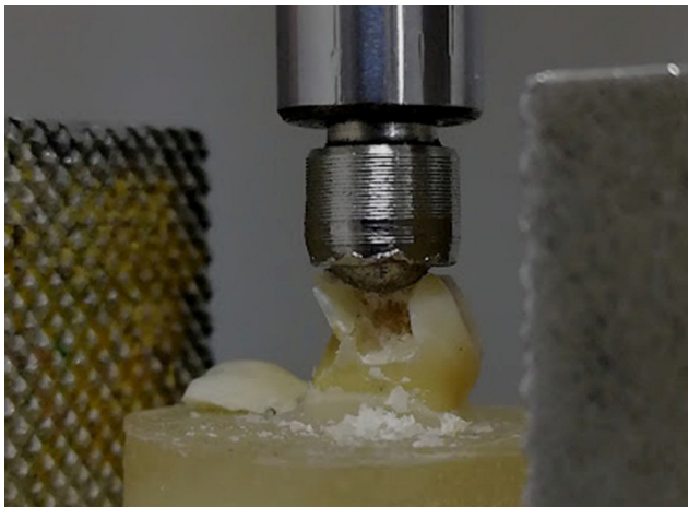
Figure 3. Catastrophic severe longitudinal vertical fractures observed in unbeveled samples.
