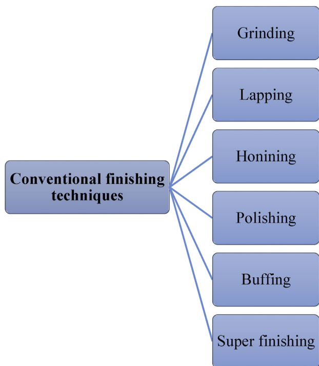
Fig. 13 – Conventional finishing techniques.
