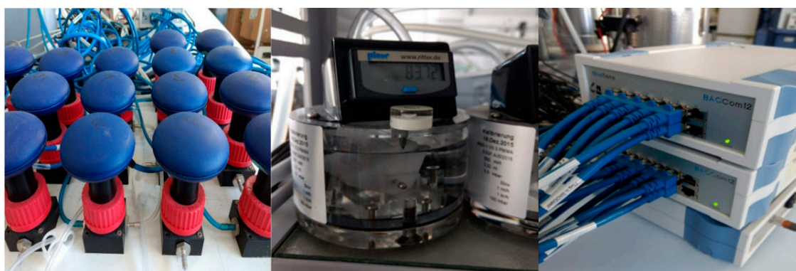
Figure 1. Equipment used for the biogas measurement and characterization. From left to right—infrared on-line sensors, the MilliGas counter, and the data interface module.
