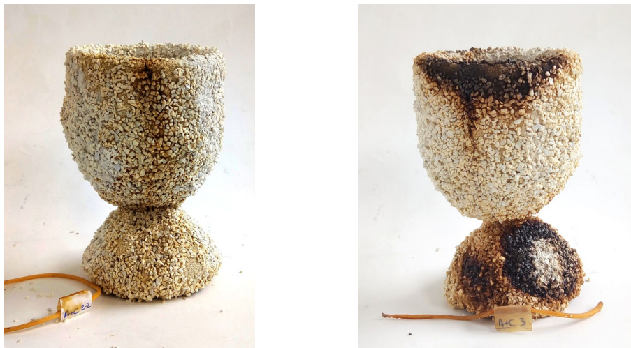
Fig. 10. Photographic record of the successful microwave dewaxing for sample 82 (left), and example of ignition for sample 63 (right).
