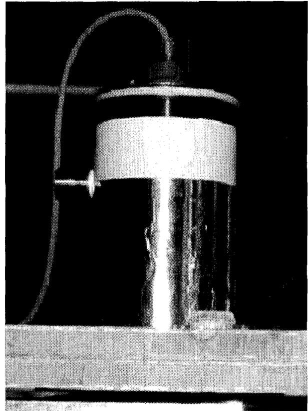
Fig. 3. A photograph of the plastic dewar and the non-magnetic frame.
