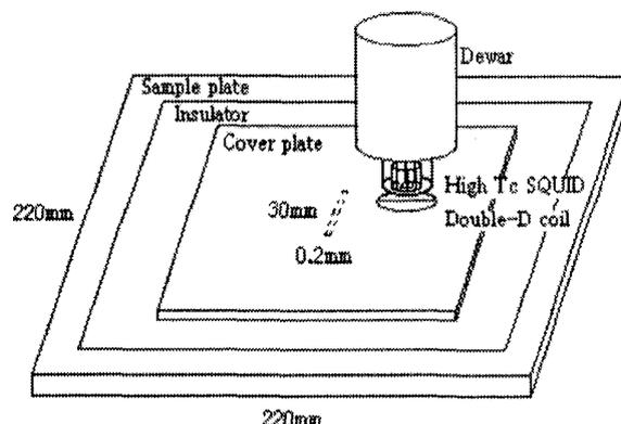
Fig. 1. The geometry of the scanning system.
