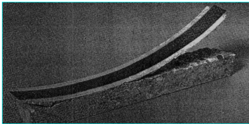
(b) Premature failure of prestressed FRP strip without anchorage
