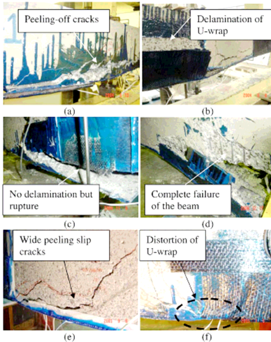
Fig.3.9 Failure modes of the beams shown in Fig.3.7: (a) J-1 with permanent metallic anchor; (b) J-2 with nonanchored U-wraps; (c) J-5 with mechanically anchored U-wraps; (d) J-6 with mechanically anchored prestressed U-wraps; (e) J-7 without side sheets; and (f) J-9 with CFRP-sheet anchor and without side sheets (Kim et al. 2008a,b).
