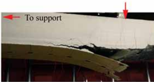
(a) Concrete crushing (Beam A-N)
