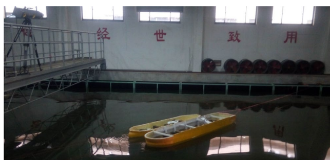
Figure 8. FPSO along with shuttle tanker model; side-by-side mooring being installed.
