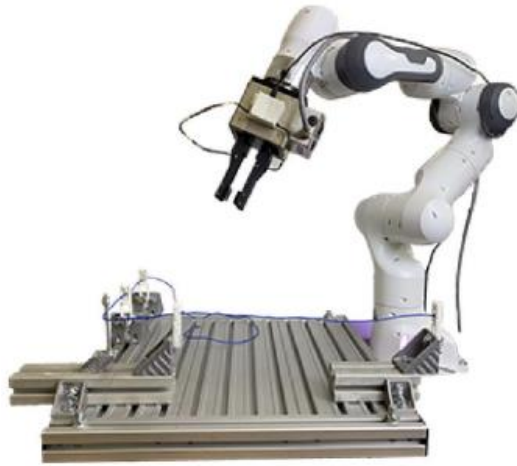
Figure 20- The cyber-physical system for cable manipulation composed by a robotic arm, a parallel industrial gripper and a pair of tactile sensors [12]
