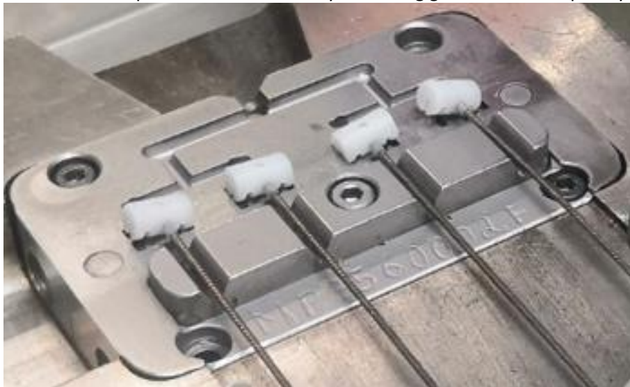
Figure 23 - Cable end Fittings Positioned in Mold After Plastic Injection
