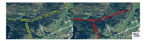
Figure 1.4: AI tool result of detection of a Power line from a satellite image *Image credit:* [31]
