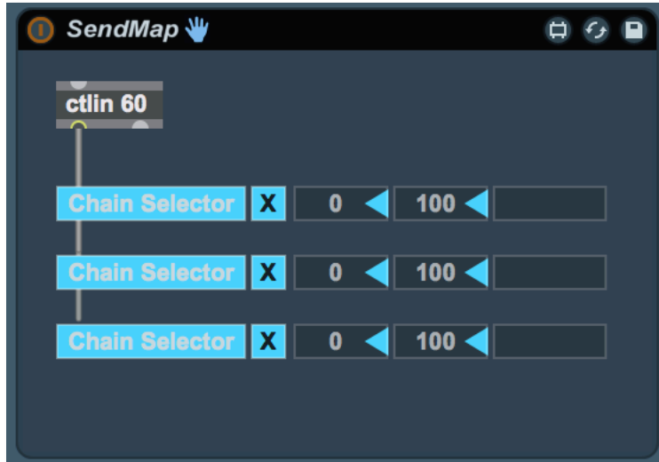
Figure 12. Max for Live device to switch the return's effects.
