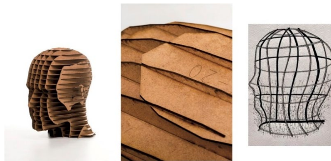
Figure 7. Digital modeling and laser cutting prototyping.
