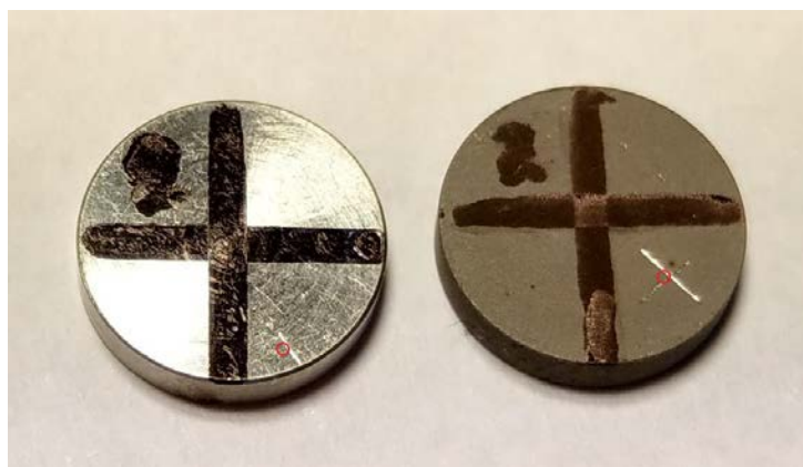
Figure 5. The two kinds of titanium discs, machined and acid-etched, used for the surface alteration test with markings to easier align the before and after SEM pictures. Figure from study I : Malmqvist et al. 2019, CC-BY.
