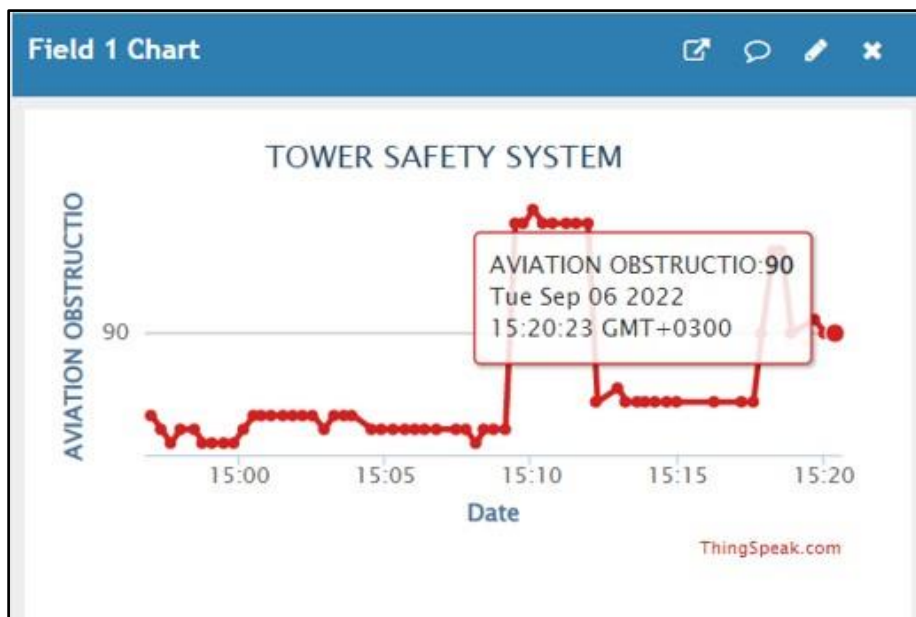
Figure 26: Illuminance of the aviation obstruction light monitoring
