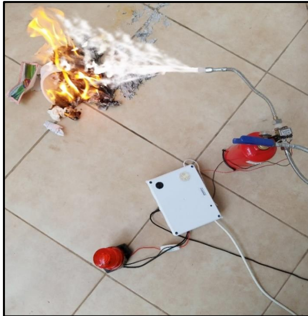
Figure 25: Detection of fire with real-time extinguishing
