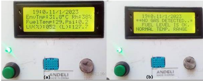
Fig. 10. LCD testing results (a) fuel data and (b) fuel condition updates to a display.
