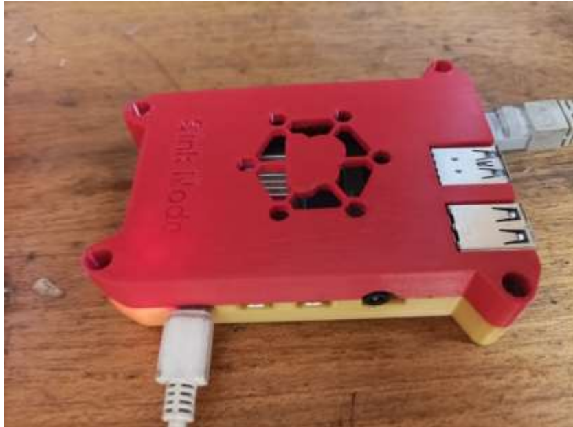
Figure 45: Raspberry pi sink node in customized 3D casing upper view
