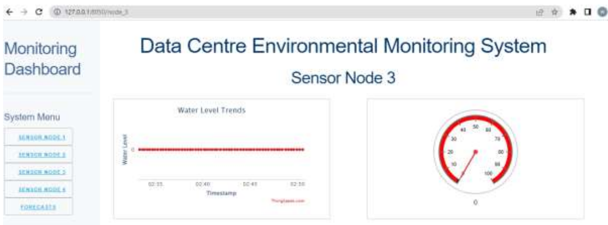
Figure 69: Sensor node 3 page displaying water level trends
