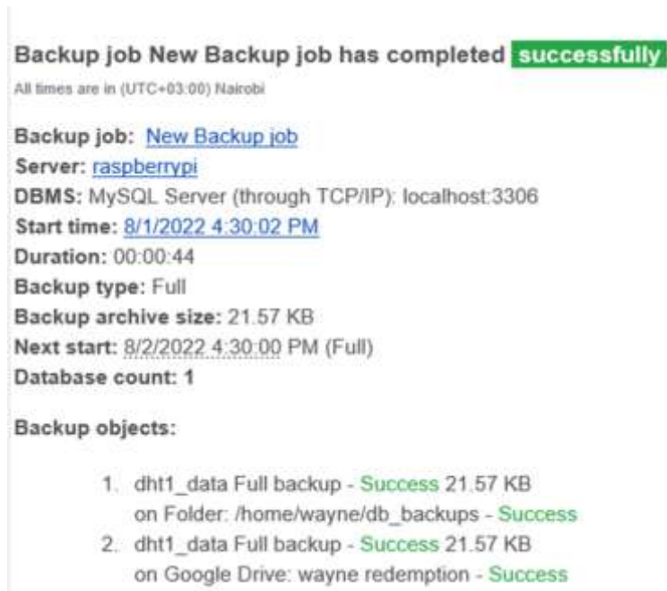
Figure 47: Confirmation message of successful database backup using SqlBak
