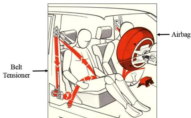
Figure 1.2: Trigger of Airbag and Belt Tensioner [2]
