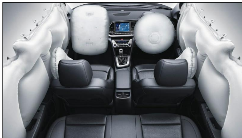
Figure 1.5: Front, Side and Curtain ABs in a Car [4]
