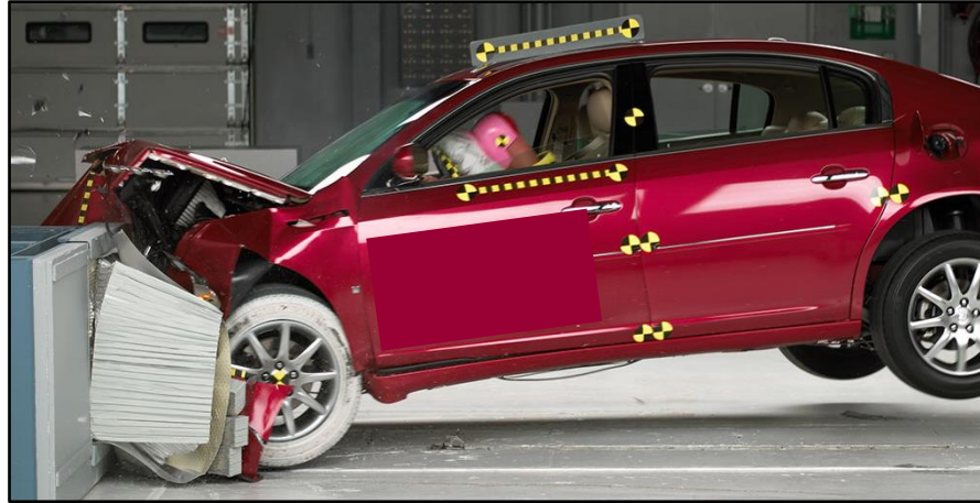
Figure 1.8: Frontal Car Crash Test [6]
