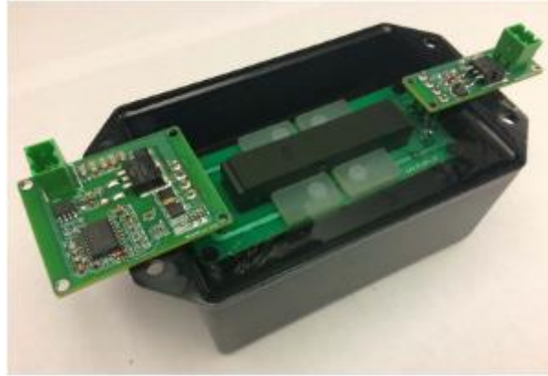
Figure 2. 23. Voltage transformer gate driver power supply with silicone gel dielectric material.
